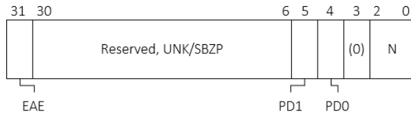
Figure 5-21: TTBCR register bit description
